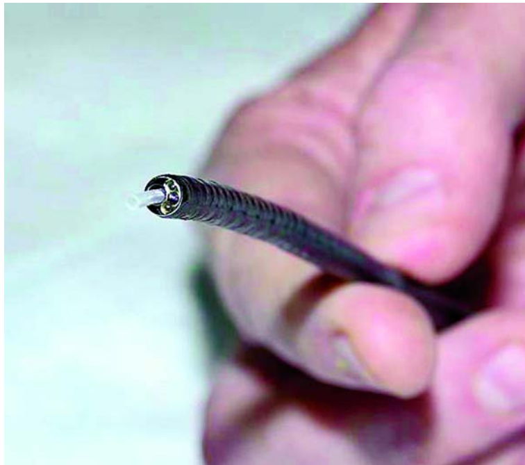
The "business end" of an endoscope has light sources and a central channel that allows the introduction of suction tubes, snares and other instruments to perform procedures without using more invasive techniques.
