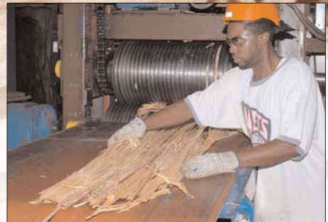
Quad Sudduth separates strands of wood in the TimTek pilot plant.
