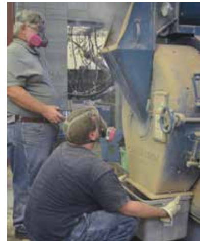
James Wooten, an Extension associate in the Department of Agricultural and Biological Engineering, monitors a pelletizer. Dr. Jason Street catches pellets to determine the machine's production rate. (Submitted Photo)
