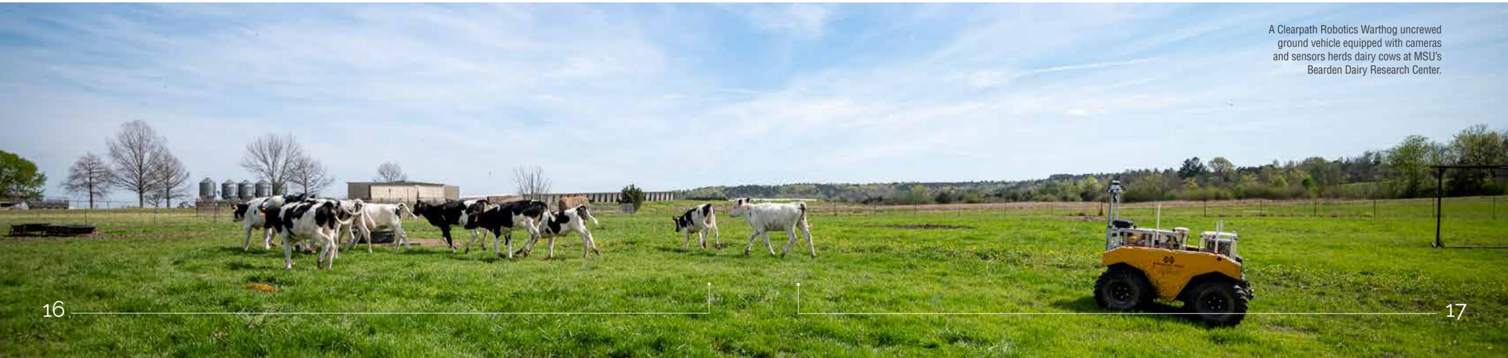
A Clearpath Robotics Warthog uncrewed ground vehicle equipped with cameras and sensors herds dairy cows at MSU’s Bearden Dairy Research Center.
